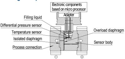
Differential pressure transmitter includes two functional units:
