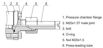
NPT1/2 male with bolts and pressure tube, SS304(Code3)
