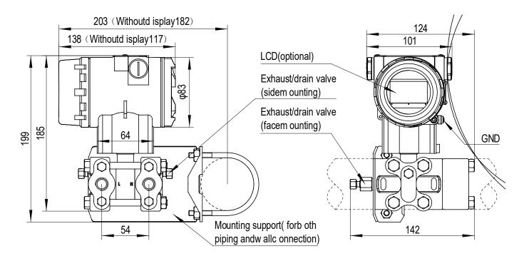
Horizontal Piping Installation (side view)
