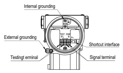
Note: the function of shortcut interface is equal to signal terminal.
