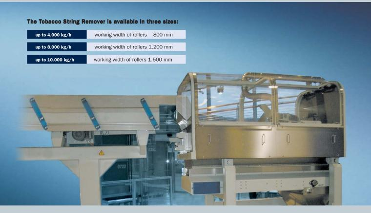
The Tobacco String Remover **TSR** is developed to remove long-fibred foreign bodies like strings or feathers from leaf tobacco and/or various blends. Cleaning of the tobacco is effected by 6/8 picking rollers lined with a food-proof "scraping" belt fitted with stainless steel pins. Foreign bodies are caught and held in the needles of the scraping belt without any damaging effect on the tobacco.
