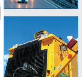
Safety: mvBlueCOUGAR-X provides more safety at construction sites. Reliable person tracking in 3D – regardless of the environmental lighting. The driver will be alerted within 300 ms after the event.
