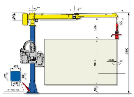
Structural versions: column mounted on fixed base-plate, autostable base-plate of our supply properly dimensioned.
