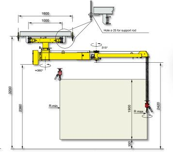
Air supply: dry and oil-free compressed air min. constant 0.7÷0.8 MPa
