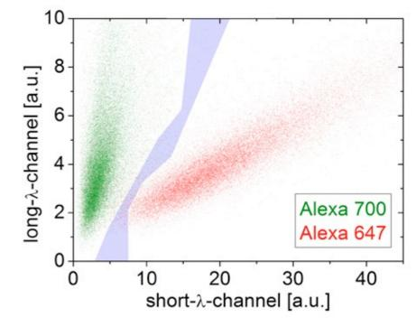
Figure 1. SD-dSTROM reconstruction of microtubules Microtubules were stained separately with either Alexa 647 (red) or 700 (green) and imaged with SD-dSTORM. The intensity values for localization of Alexa 647 (red) and Alexa 700 (green) show different populations in a 2D intensity histogram. The intensity-based color assignment filter discards localizations in the cross-talk region (grey).
