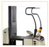
Lifting platform and picking guard (GPC 3040/3060)
