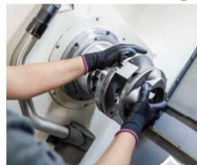
I insert the jaw module, secure it with a screw and it is already centered. Everything is ready in no more than 2 minutes. Clamp the workpiece and machine it from all sides, or between the jaws. But the best part: I don't have to change over to an entire jaw chuck.
