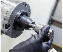
If you have a part you want to machine over the entire length, for example, you can use the face driver for machining between centers. I know I have already mentioned this several times, but this too takes less than 1 minute, and no alignment is necessary.
