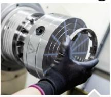
This allows axial machining of the part on a neodymium magnet, and the magnet module is pulled onto the flat contact face on the basic clamping device. You already know: 30 seconds, and no ...
