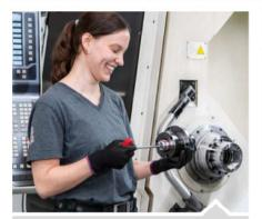
As you can see, I have already removed the clamping head from the chuck. While holding the MANDO Adapt T211 adaptation in my hand, I insert the segmented clamping bushing and then tighten the draw bolt.
