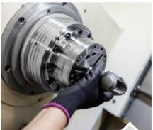
Not only is the system very fast, but requires no alignment. Now I can clamp the workpiece to be machined from the outside and start the machine. One more tip: High machining parameters are no problem thanks to the unique rigidity of the system.
