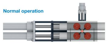
The heated steel housing allows for two screen bearing pistons, positioned transversely to the melt stream, and containing two screen cavities each per piston. The melt flow is subdivided into four flow paths, directed through each of the four screen cavities, and reunited after filtration at the material outlet. The contamination of the melt and the resulting deposits on the screen packs result in an increase in flow resistance.
