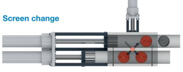
The screen change takes place when the self-cleaning is completed. The screen piston with the filter element to be cleaned is moved out of the housing, far enough to allow for the screen pack to be removed and replaced with a new filter element. During the screen change, three screen cavities (75%) remain in production. The screen change proceeds for all four screens successively.
