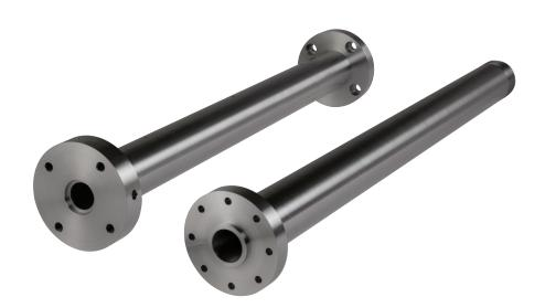
**Strong and straight.** The structural shell of Xaloy bimetallic barrels consists of a microalloy steel that maintains high strength and straightness after casting of the wear-resistant alloy lining. Unlike some barrel manufacturers, Nordson can produce long barrels – up to 240 in. (6.1 m) – without resorting to butt welding. The benefit to you is a stronger, straighter barrel with no seams to trap polymers that can degrade and contaminate your process.
