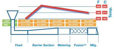
Nordson recommends that a "hump" type barrel zone temperature profile be used to optimize the performance of the Fusion™ Screw. Make sure that you request the best temperature profile from your Nordson representative for your resin and process.
