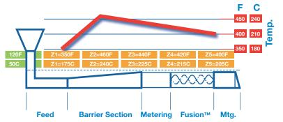
Nordson recommends that a "hump" type barrel zone temperature profile be used to optimize the performance of the Xaloy Fusion  $^{\text{TM}}$  II screw. Make sure that you request the best temperature profile from your Nordson representative for your resin and process.
