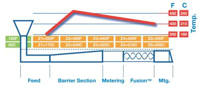
Nordson recommends that a "hump" type barrel zone temperature profile be used to optimize the performance of the Xaloy Fusion™ II Screw. Make sure that you request the best temperature profile from your Nordson representative for your resin and process.
