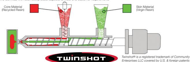
Available only from Nordson, Xaloy® Twinshot® enables a conventional machine with a single barrel and screw to inject two materials in one operation, with one material totally enclosing the other.
