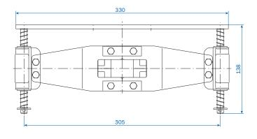
max. horizontal offset 10 mm max. vertical offset 10 mm
