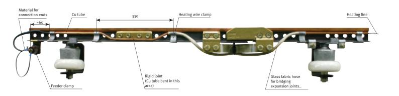
Installation (and retro-fitting) is also possible on conductors which have already been installed, as the copper tube is fixed using galvanized spring clamps. Rigid and expansion joints are bridged according to the illustration.
