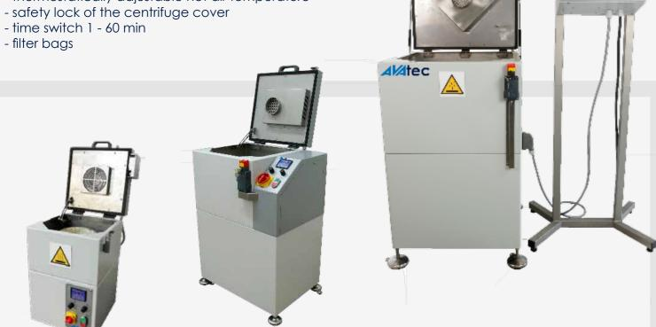
Bulk materials as well as sensitive parts can be dried in the centrifugal dryer Special versions of baskets, sieves and adapter on request
