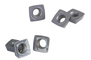
The new designed QUADWORX® indexable inserts have 4 cutting edges and a special geometry, a combination of large corner radius and wiper edge. This ensured best performance in 2, 2 1/2 and 3D cutting. For increased tool life, all cutting edges were edge-treated and polished to reduce the friction between cutting material and insert.
