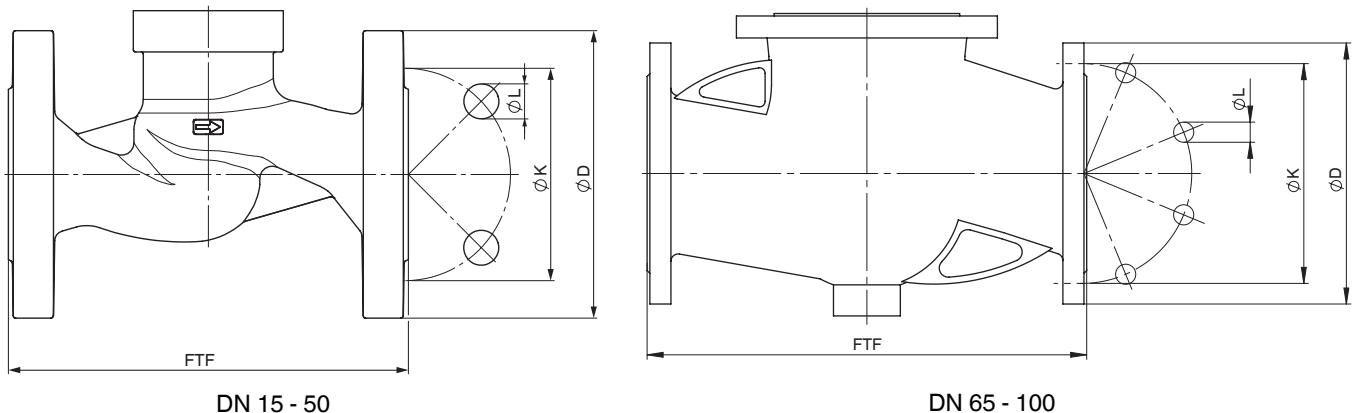
Connection type flange, length EN 558 (code 39)<sup>1)</sup>, investment casting material (code 37), SG iron material (code 90)<sup>2)</sup>
