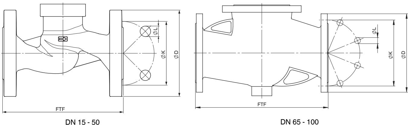
Connection type flange, length EN 558 (code 8)<sup>1)</sup>, SG iron material (code 90)<sup>2)</sup>
