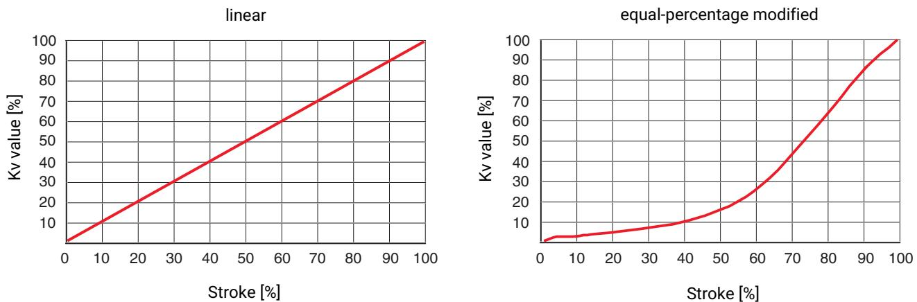
The diagram shows the approximative curve of the Kv value characteristic. The characteristic may deviate depending on valve body, nominal size, regulating cone and valve stroke.
