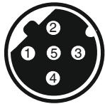
5-pin M12 built-in socket, D-coded
