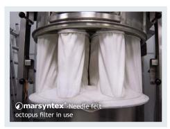
marsyntex° filters for fluid bed driers can be produced in different sizes and with up to 98 sleeves. Furthermore, we offer these in an anti-static fabric or needle felt with a different separation efficiency and different surface qualities.
