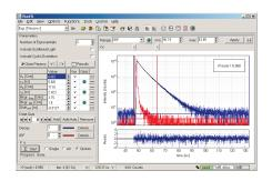
Various exponential decay models (up to fourth order) or rate constant distribution models can be fitted to the observed decay. FluoFit also supports the analysis of anisotropy measurements as well as global analysis for all methods. Running FluoFit simultaneously with the measurement software allows for parallel data analysis.
