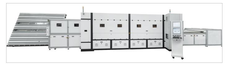
Using ultra-short laser pulses, the CLT 8oG cuts by material disassociation rather than ablation. The result is a very low surface roughness, increased as-cut edge strength and faster throughput. The Corning Laser Technologies process enables cutting fully strengthened glass, Corning<sup>®</sup> Gorilla<sup>®</sup> glass, un-strengthened glass, as well as other transparent glass and crystalline materials.
