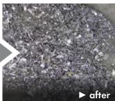
Turning – milling – drilling - is machining aluminum your profession? Then you can do without costly and time-consuming chip crushers in conjunction with lifting systems. The  $SZ_{CUT}$  combines a proven centrifugal pump design with a cutting element and optimizes the difficult transport of aluminum chips in the coolant cycle. At the suction opening
