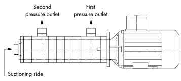
Fig.: Pump type ZHB 32-08
