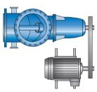
Motor to one side on a tensioning bar
