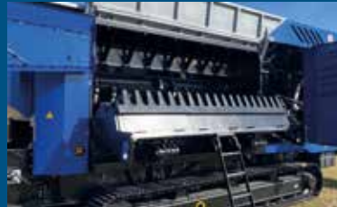
Shredding flap - can be deployed hydraulically = free access to shredding area
