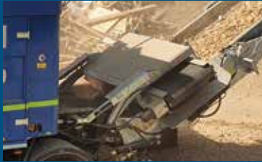
Powerful neodymium magnetic separator, hydraulically height-adjustable, scrap ejection on both sides
