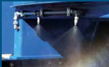
Material moistening device - for dust containment
