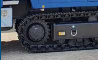
Robust tracked drives, 2 speeds, ground protection plates
