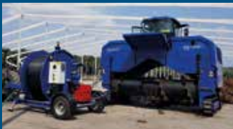
Irrigation with hose drum waggon
