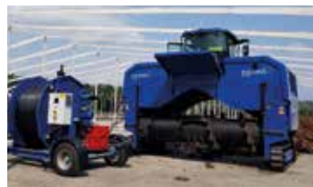
Irrigation with hose drum waggon
