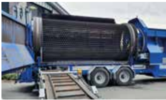
Trommel changes are easy for trommel diameters of up to 2,000 mm
