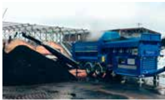
Extended fine grain belt, discharge height of up to 3,700 mm
