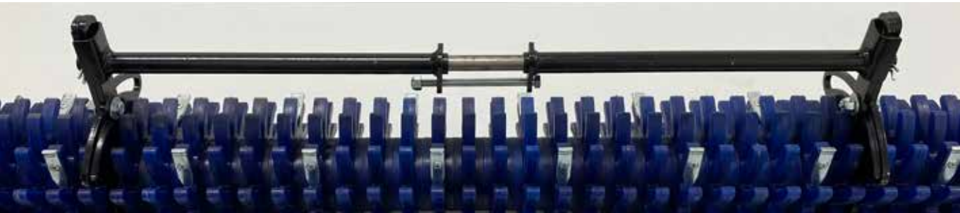
Eggersmann fine screening shaft with QuickChange system
