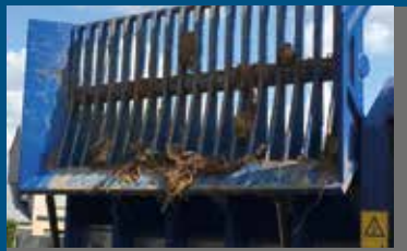
Coarse material separator - to protect the bunker in case of large impurities
