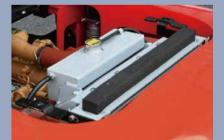
A plate-fin heat dissipater with high-performance fins is used to enable low oil and water temperature without water and oil leakage
