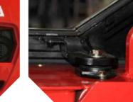
There're four levels shock absorption applied to reduced the vibration from the road to the driver. The damping pad is applied reduce the vibration, Like between the steering axle and the chassis, The engine, torque convertor and the chassis, the overhead guard and the chassis. And the suspension seat is another vibration reduction.
