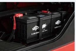
The battery is located above the fuel tank, there's battery box and adiabatic plate between them to prolong the battery's workling life.
