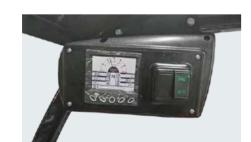
Interactive instrument: The instrument adopts LCD display with four interactive buttons, and has one CAN bus communication function. The communication protocol is compatible with CANopen and SAE J1939 standards.
