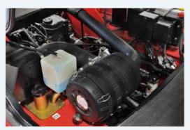
The new stamped air cleaner featuring tangential intake, double seal with safety filter is durable, corrosion-free and vibration-resistant, provides better filter efficiency and lower intake resistance than the previous.
