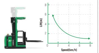
A smart driving deceleration system is used the driving speed is related to the lifting height. The high<mark>er the lifting height, the lower the driving</mark> speed and the smaller the acceleration. The function of proportional speed reduction in corners is equipped as standard to ensure smooth and safe turning of the vehicle.
