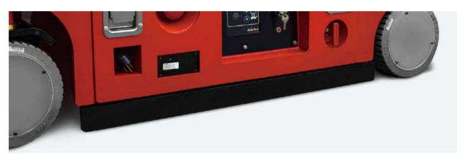
Anti-overturning system, When the machine raises to more than 2m, this system will work automatically, to protect the machine from overturning while walking at un-leveling ground
