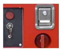
Manual lowering handle, When the operation system failed or the battery power is too low to let the platform decline, we can use this handle to lower the machine
