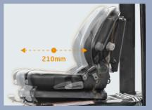
The seat can be adjusted back and forth by 210mm
