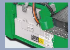
I he packs can be easily removed by a manual or electric cart, and can be repaired and maintained conveniently
