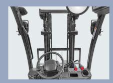
The wide-view mast with optimized design is unlikely to obstruct the operator's line of sight. The enlarged opening size of the fork carriage enables wider view. The high fulcrum of the tilt cylinder enables better force bearing and more stable operation of the mast
