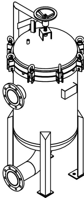
Eye bolt closure with lifting and swiveling device
