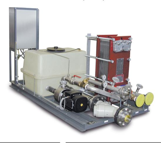
The process water treatment unit PWA serves for filtering, tempering, and circulating the process water in compound and masterbatch production and can be integrated into the base frame of the cooling trough or positioned externally. Using a heat exchanger, the PWA separates the contaminated process water circuit from the primary cooling circuit from the central water supply.
