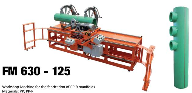
The machine is composed by a support frame with two self-centering clamps that are free to slide independently along the whole length.
