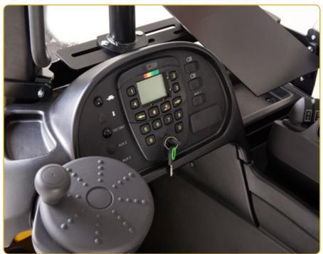
The steer positioning sensors provide feedback of the actual steer position. The standard steering has a 180° steer angle, a 360° option is available and enabled by the VCM software. A third option allows switching from 180° to 360° by pressing a steering mode selection switch on the dashboard. Speed reduction on cornering is automatic and can be adjusted.
