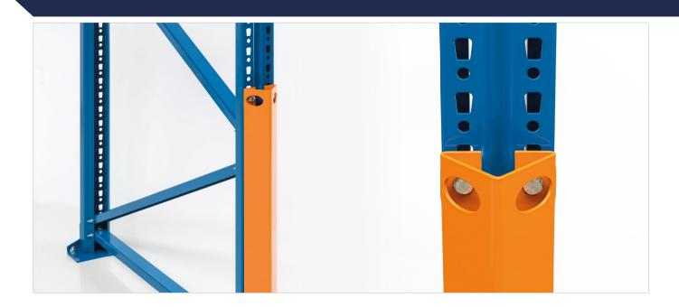
Like a shin guard, the stiffener absorbs the impact when a forklift truck - easily weighing in at 4.5 tons - accidentally collides with a rack. The length and profile have been designed to ensure that the force of the collision is optimally distributed in the rack, thus minimising damage. The connection between the stiffener and the upright is equally ingenious: the bolt holes are integrated into the profile in such a way that they are almost impossible to tear or break. Another major advantage.
