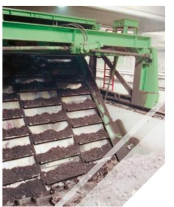
The Biofix turning machine starts from the discharge traversing system and moves to the waste material on the top of bin walls via rails.
