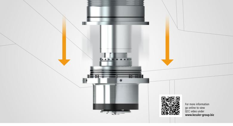
The spindle housing rests during the change in the headstock of the machine
