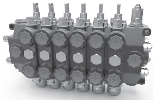
**MRS120** control valve belongs to the range of sectional MRS series valves. It is designed with an open center and is capable of working with a maximum flow 120 lpm. The valve can be used in different systems for parallel circuits, numerous valve configurations make it flexible to the wide application range.
