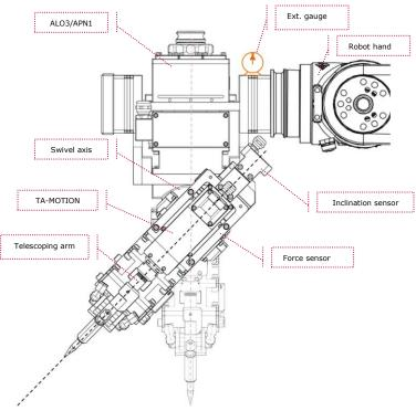
Figure 1: Actuator/sensor modules on the ALO3 processing unit
