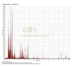
Highly resolved spectrum of a steel sample Resolving power 9,000
