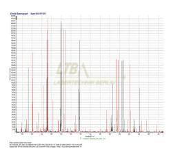
Part of a spectrum of a glas sample Resolving power 9,000
