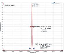
Spectrum of an excimer laser ArF 193 nm
