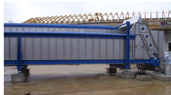
Solid material metering feeder 40m³ ceiling installation
