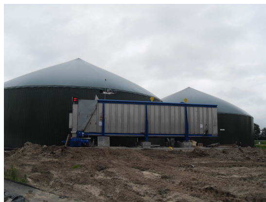
60 cbm feeder with method for injection below liquid (up to 6 m under water)
