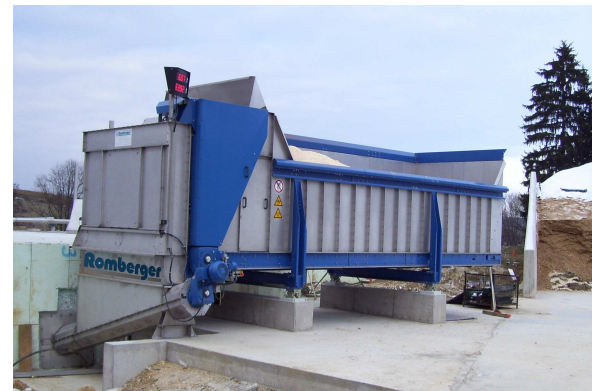
30 cbm metering feeder with lateral fermenter screw Scraper floor version with closed underfloor
