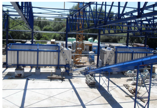
Solid material metering feeder 2 x 50 m³ performance 210 to/d
