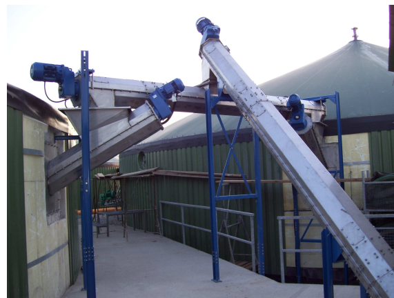
Inclined screw conveyor with distribution over two fermenters.
