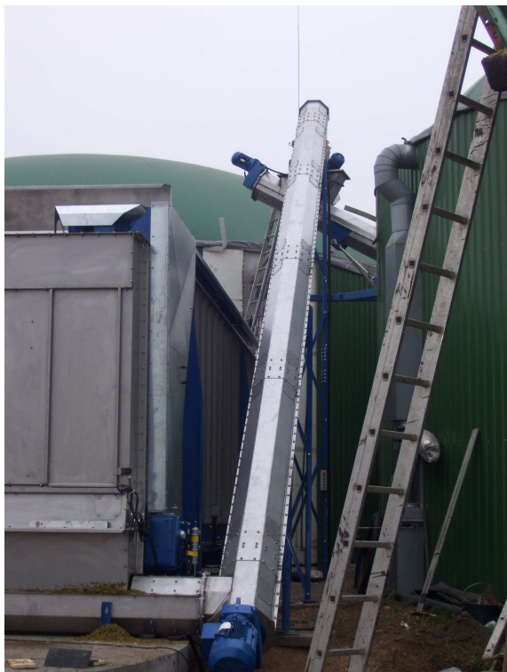
Metering feeder 50 m 3 with inclined screw conveyor and two fermenters.
