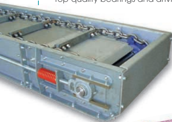
Double line trough scraper with rounded link chain for rock pieces, tensioning station with spring pre-stressing
