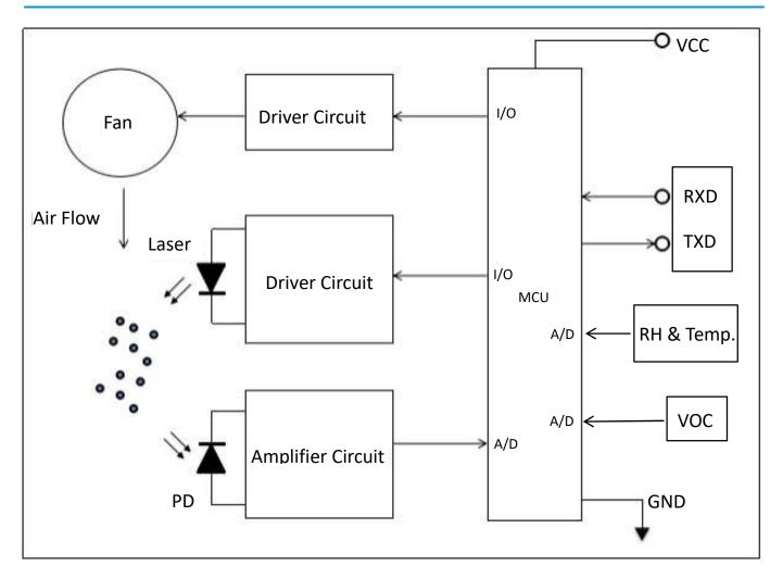
According to the above figure, the light source part of AM1002 is composed of a laser tube and a driving circuit. The detection part of the sensor is composed of light sensitive part which receives reflected light and amplifying circuit. Data processing and communication output are completed by microprocessor.
