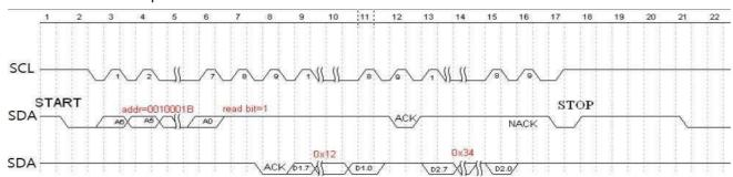
Picture 7: The master device receives the data from the slave device
