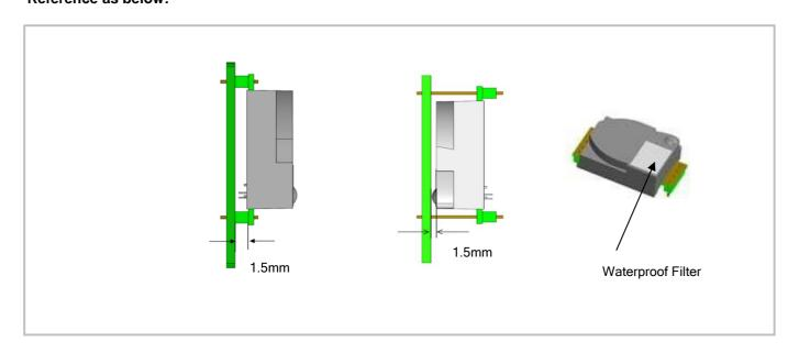
2. To avoid the influence of stress on sensor, please soldering by hand as much as possible when mounting the sensor to the PCB.
