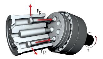
The large, non-compensated forces in bent-axis motors need to be absorbed by extra-large ball or roller bearings. This increases the space required in the machine and makes integration more difficult.
