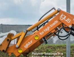
heavy-duty test with a maximum load of 500kg From more than 15,000 tests performed per year, we have created what is probably the wor-Id's largest test database. This database gives us the ability to always select the right product for your specific application. Individual tests for your industry are also possible.
